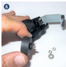
Diaphragm is removed from the magnet bracket
