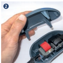
Pump cover is removed
