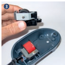
Unscrewing the air chamber and removing it from the housing
