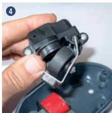
Removing the diaphragm from the air chamber
