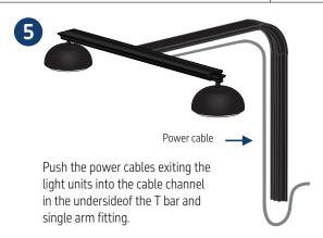
T bar then tighten screws.
