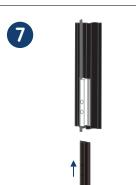
Slide the bottom of the single arm fitting into the arm mounting track and push the bottom section of power cable into the recess.
