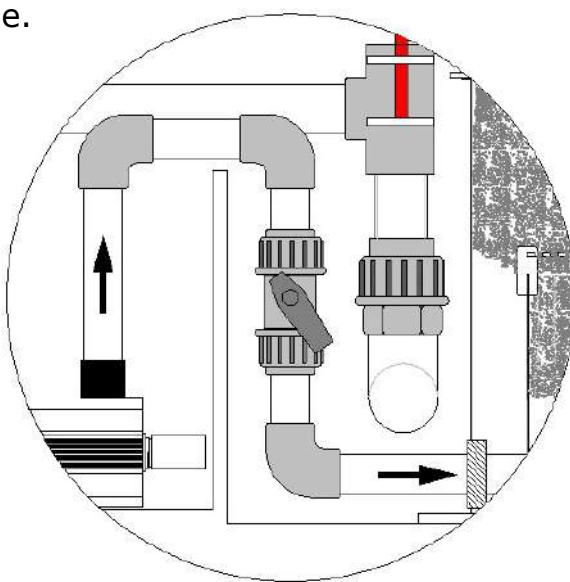
d) Shut off valve inlet
